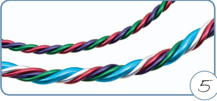
5- Unhook the wire from the wire twister and cut the parts that are not twisted.
